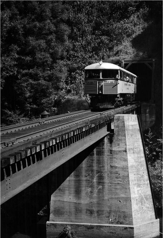
Our gas-powered, self-propelled M-100 railcar (a 'Skunk') in the 1960s
